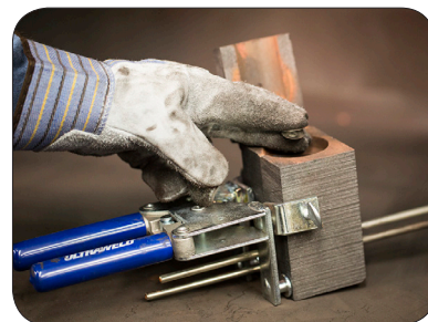
Step 3: Insert disk into mold.
